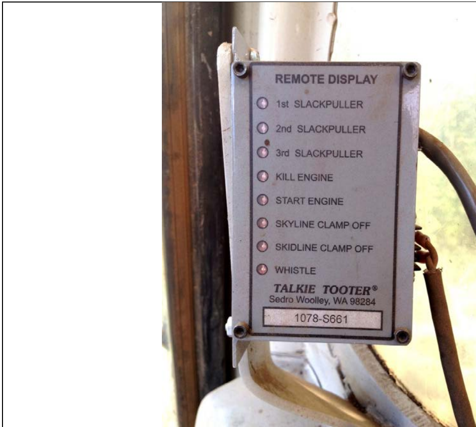
One of the control panels in the cab of the yoder. Casey d'Agostini, Jr., the operator communicates with the timber faller and riggers downslope by whistle combinations.
