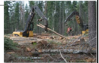
Figure 3. Fellerbuncher and skidder.
