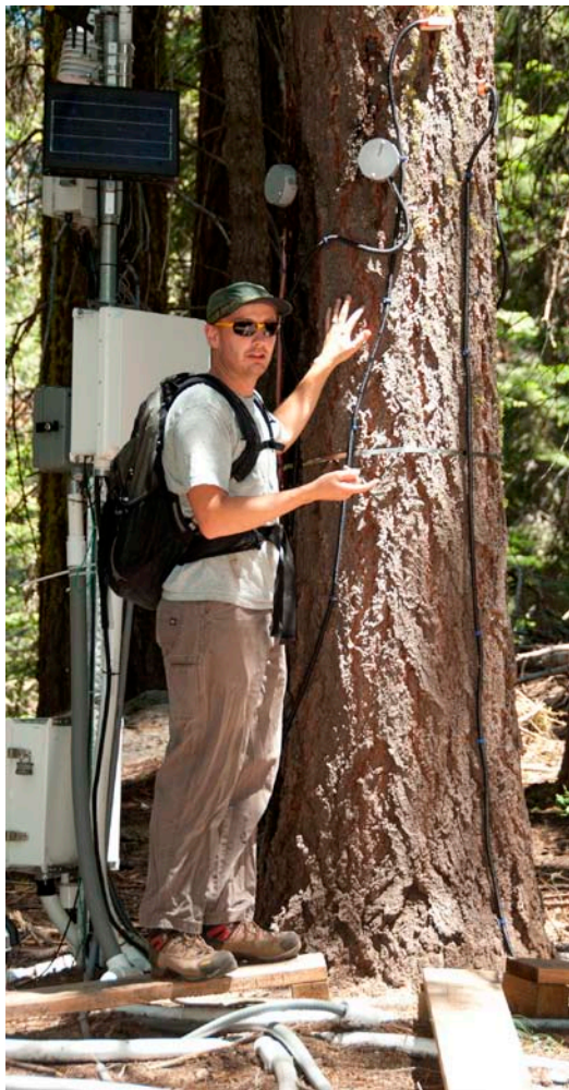
Figure 5. UC Merced hydrologist Matt Meadows shows off the sap flow meters in a white fir on site. Photo by Sharon Eng, USFS PSW.
