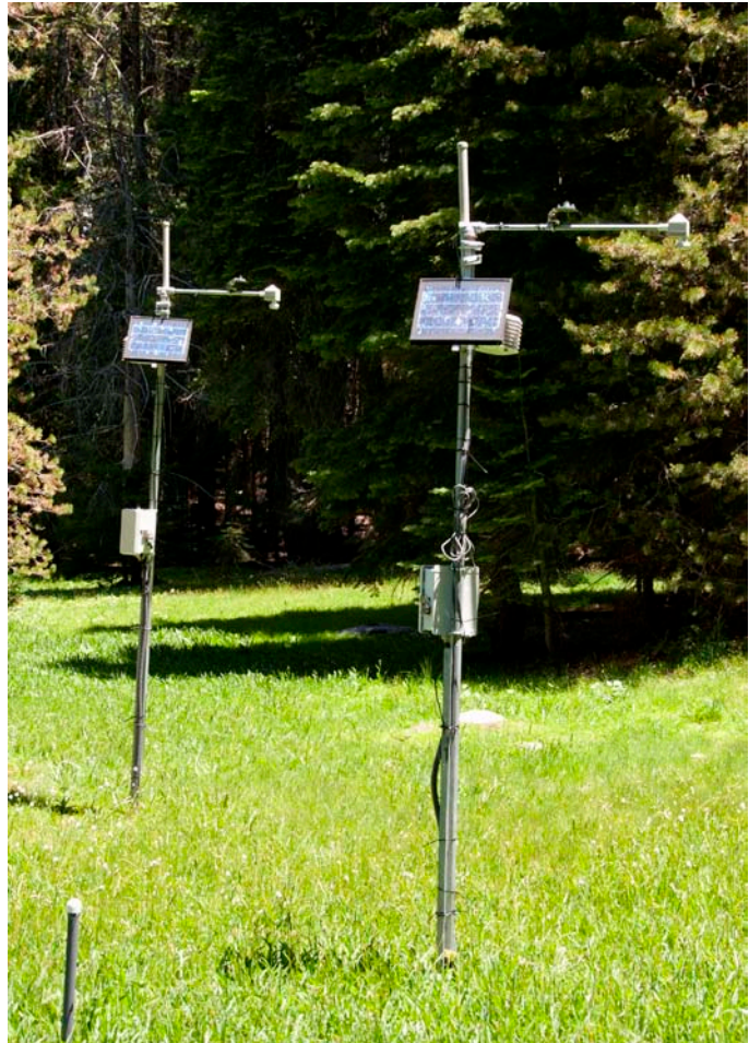
Figure 6. Wireless monitoring stations in meadow. Photo by Sharon Eng, USFS PSW.
