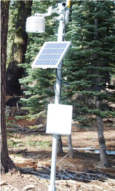
**Figure 2. Snow depth sensor at Duncan Peak.**
