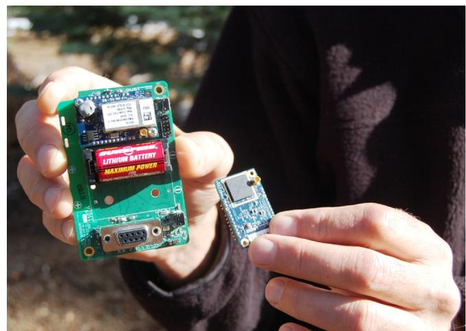
**Figure 3. Low power computer components used in the sensor wireless system.**
