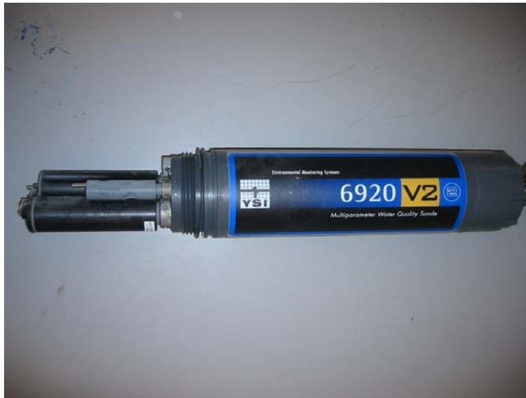
Figure 4. YSI 6920 Water Quality Monitoring Sonde
